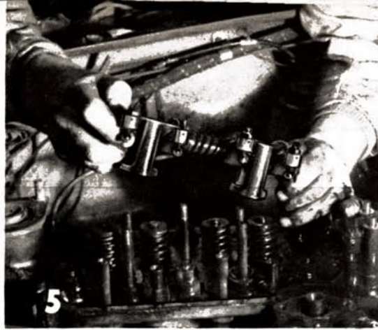
When removing the rocker gear, take care not to lose the two washers which lock the nuts. Be gentle with the pushrods, too.
