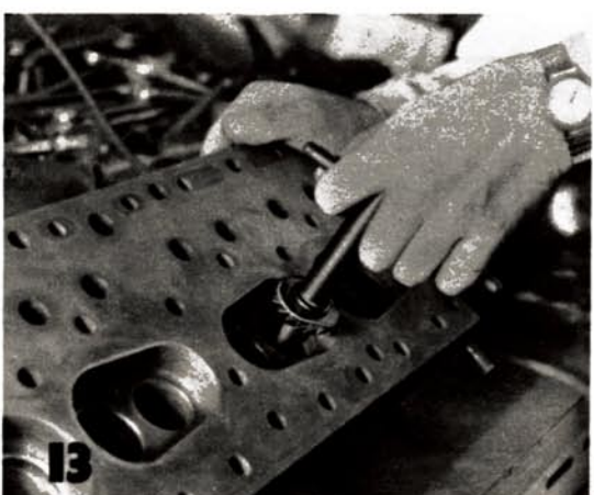
Really bad valve seats, such as that shown on this page, can only be treated by using a 45-degree cutter, to make a fresh seat.
