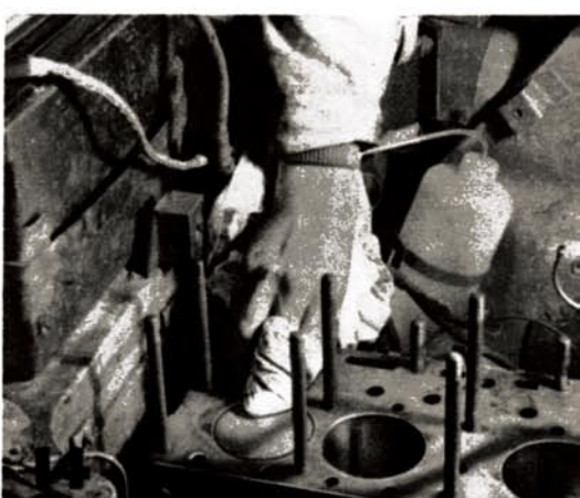
The pistons need not be taken out. Scrape the carbon off the crowns and then finish the job with metal polish. Wash with petrol.
