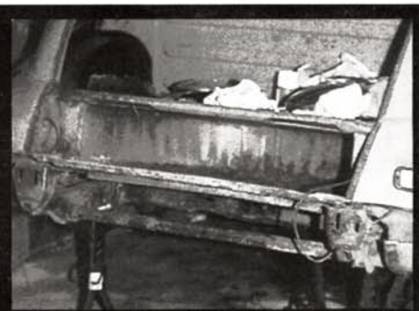
● The rear ends can be devastated by rust extending from the boot to the fuel tank.
