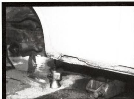
● Sills are rust-prone areas as are the rear wheelarches.
