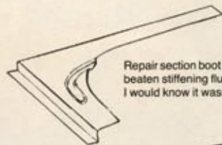
Spare wheel compartment hand formed from one piece.
