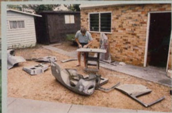
Bob was careful to take all the panels back to bare metal before they were primed. All repairs were made with oxy-acetylene welding equipment.
