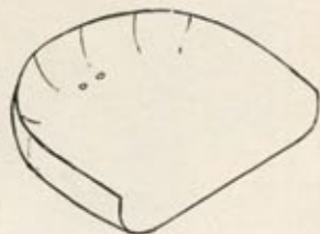
A front floor repair piece used simple press forming tools to produce stiffening flutes.
