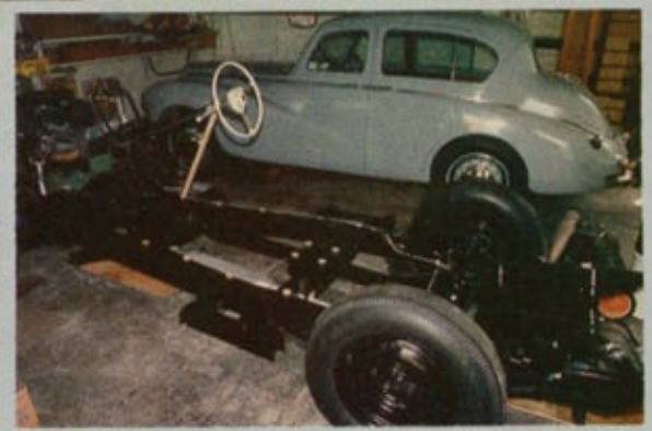
The chassis was repaired, chromated and black-enamelled to the original specification, then fitted-up and used as a static display at the Melbourne British Motoring Show.
