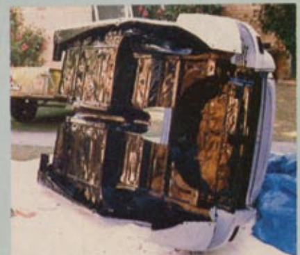
Replacement floor and door sections and a spare wheel well were made and fitted. The whole body was sand-blasted, inside and out, and the underside painted.
